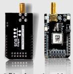
"tGPS BoB" is a formative with a microBUS structure. It is an effective and easy solution for adding GPS functionality to your design. It features the Telit SL871 module, a SMA connector for a GPS antenna also it has two LEDs for PPS and PWR. tGPS BoB can be interfaced with the target board microcontroller via microBUS UART (Rx, Tx), lines. It has a LED diode in order to power indicator. It can function on 3.3 V power supply only.
